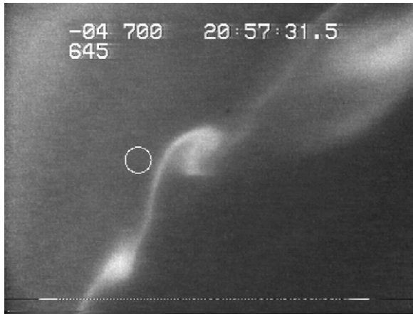
Fig. 8. EISCAT field of view compared to the width of a filament. The field of view is 38 \times 28 km; north is to the right and east to the top. The circle gives the field of view of both EISCAT and a photometer. Its diameter is about 900 m. Neither of these instruments can thus directly resolve the 100 m wide filament (from Lanchester et al., 1997). Reproduced by permission of American Geophysical Union.
