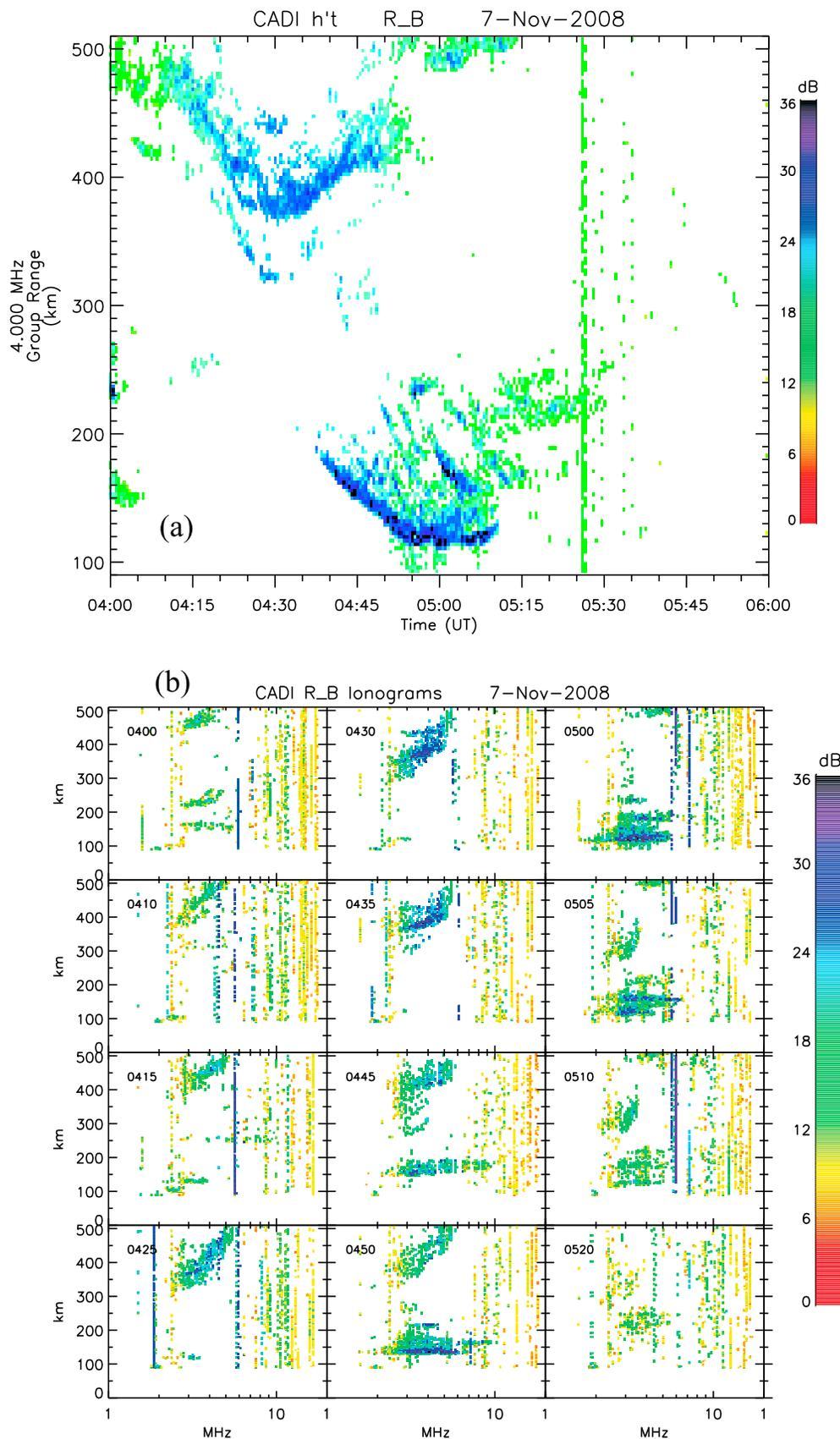
**Figure 4.** Resolute Bay Canadian Advanced Digital Ionosonde (CADI) (a) measurement of group range at 4 MHz for the period of 0400–0600 UT of 7 November 2008 and (b) sequence of 10 min interval ionograms between 0400 and 0520 UT.
