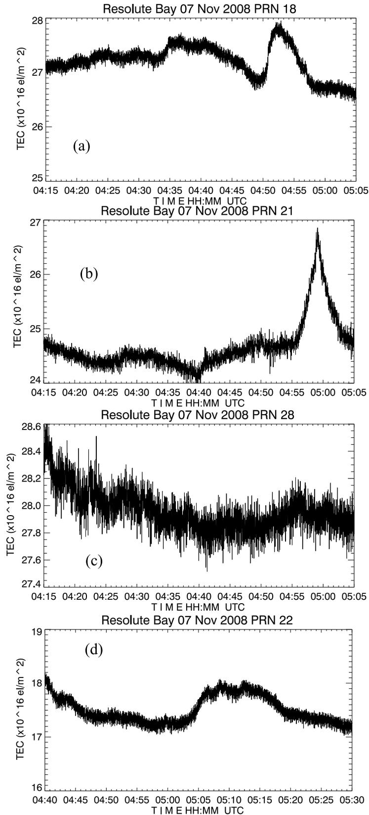
**Figure 3.** Variations of relative total electron content (TEC) along the raypaths of GPS satellites (a) PRN18, (b) PRN21, (c) PRN28, and (d) PRN22 for 7 November 2008 at Resolute Bay. Note that Figures 3a–3c are for the period 0415–0505 UT and Figure 3d is for the period 0440–0530 UT.
