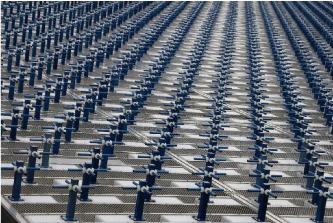
**Figure 2.4:** Image of individual antenna element units (AEUs) on the face of the RISR-C radar. Image from Gillies & Varney (2016).
