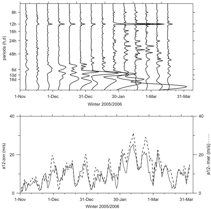
Fig. 5. Long periodic oscillations of meridional winds (upper panel) and semi-diurnal tidal components (lower panel; full line: zonal component; dashed line: meridional component) derived after meteor radar observations at an altitude of 82 km at Andenes in winter 2005/06.
