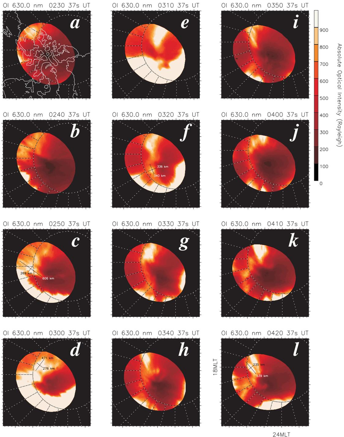
**Figure 2.** Sequence of 630.0 nm airglow images at 10 min intervals from 0230–0420 UT.
