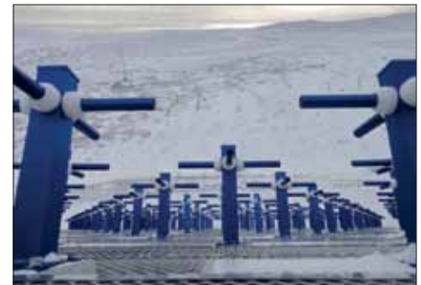
1 (Left): North face of the Resolute Bay Incoherent Scatter Radar (RISR-N), which probes the plasma parameters in the polar cap ionosphere, and (right) crossed dipole antennas on RISR-N. (C Heinselmann)
